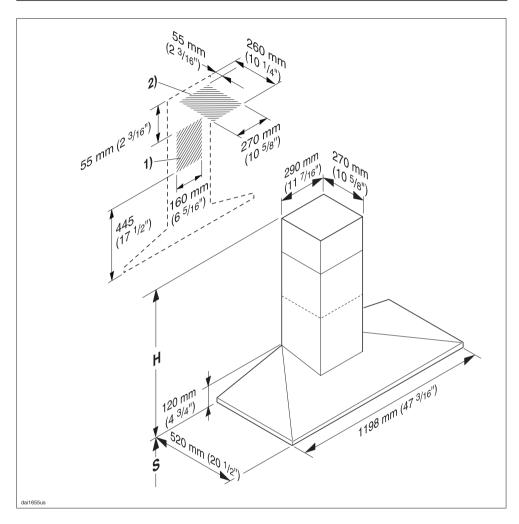
1) and 2) Installation area Wall/ceiling area respectively for vent hole and outlet installation.
